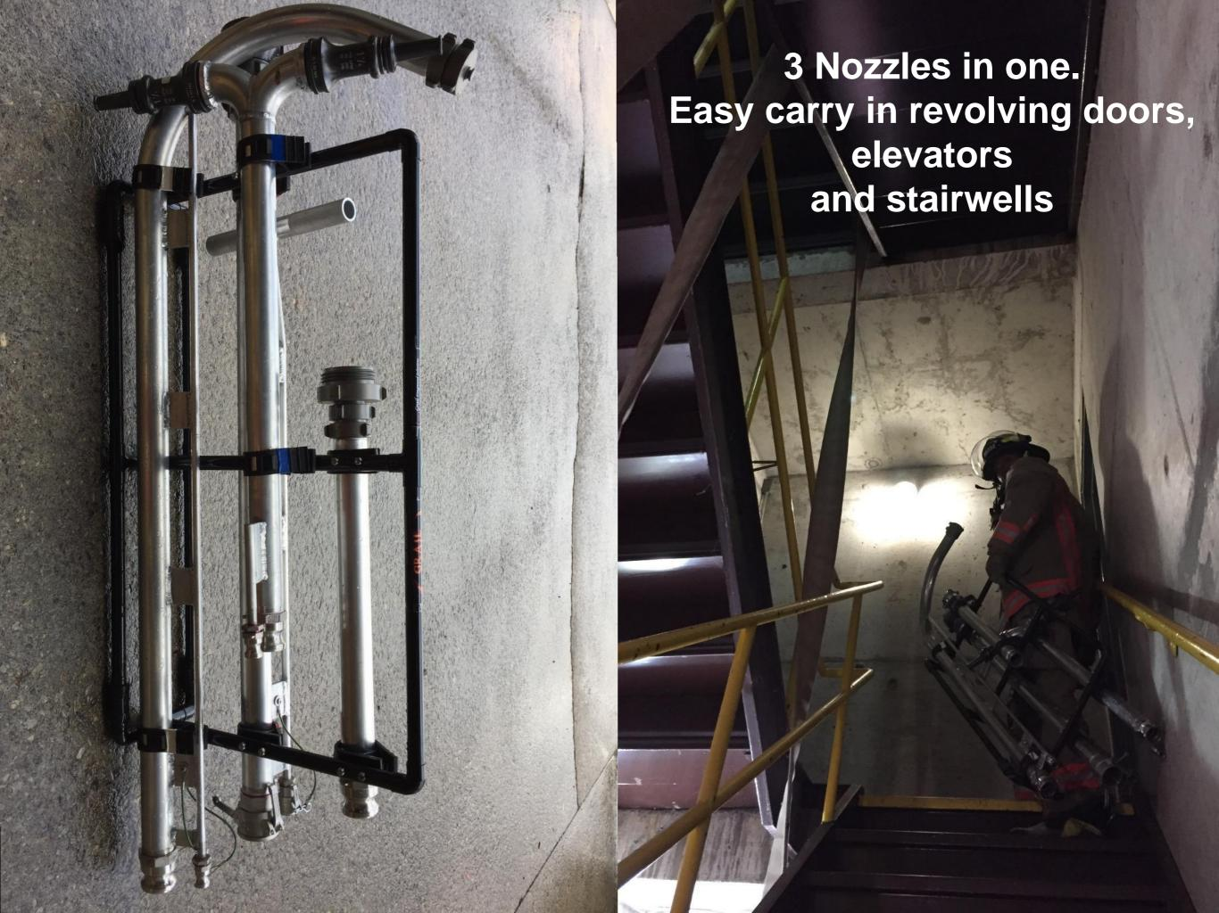
Floor below nozzle used for wind driven fires
